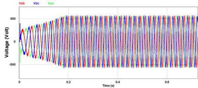
Figure 14. Output voltage from the inverter
