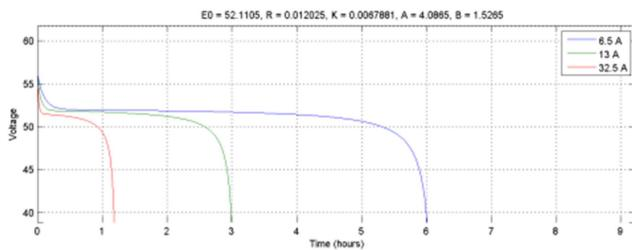
Figure 8 characteristics of the battery discharge with different discharge currents
