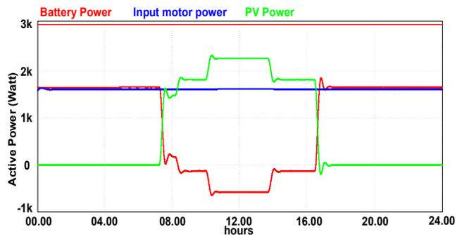
Figure 16. Curve shows the relation between PV power, Battery power and motor absorbed power within 24 hours.
