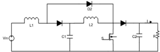
Figure 3 Circuit scheme of quadratic boost converter
