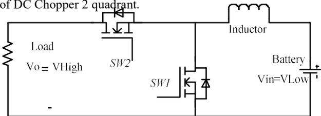
Figure 4 Two quadrant DC-DC chopper
