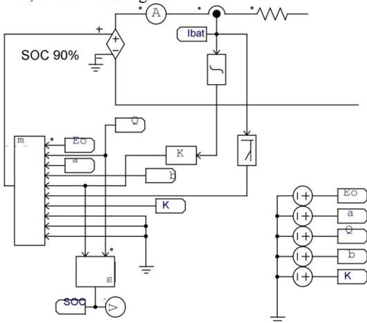
Figure 9. Modeling battery on PSIM
