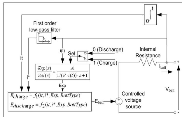
Figure 7. Schematic model of battery on MATLAB
