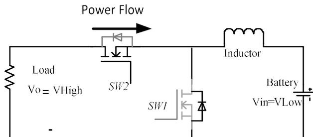
Figure 6. Buck mode from bidirectional converter
