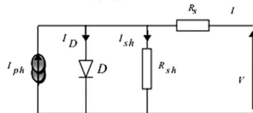
Figure 1. PV equivalent circuit
