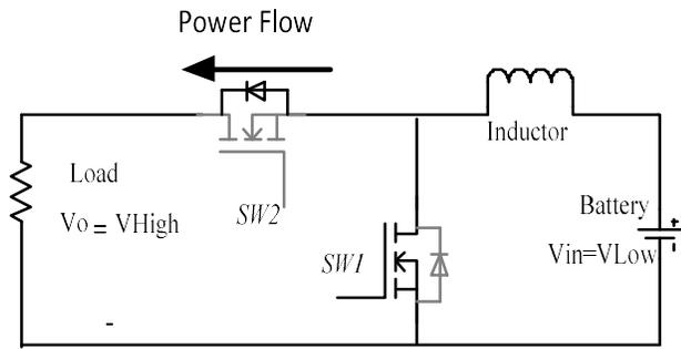
Figure 5 Boost mode from bidirectional converter
